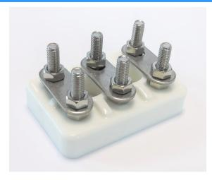
These terminals allow the connection star-delta three-phase motors or two separate motors. Thanks to the excellent thermal resistance properties conferred by ceramics, they find application in machinery such as electric ovens, motors with high operating temperatures, equipment where very high temperature resistance is required, such as smoke and heat extraction fans. These terminal blocks are also used for star-delta switching of three-phase heaters.
