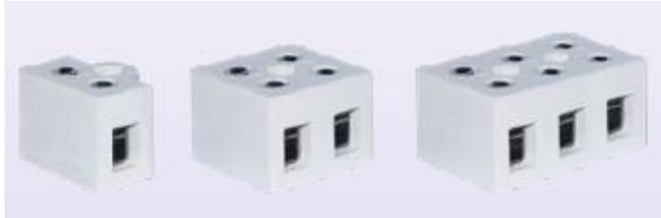
Terminal blocks one, two and three pole (pin) in technical ceramics. Impressive properties and resistance to high temperatures of ceramic enable to apply this type of terminal blocks in electrical devices for both industry as well as domestic users. In the industry field are used in extremely high temperature applications such as furnaces, heaters, process equipment and machinery, road tunnels, train and subway tunnels and for parts of vessels that must resist fire.
