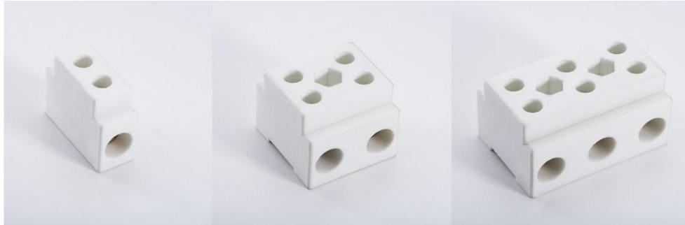
Terminal blocks one, two and three pole (pin) in technical ceramics. Impressive properties and resistance to high temperatures of ceramic enable to apply this type of terminal blocks in electrical devices for both industry as well as domestic users. In the industry field are used in extremely high temperature applications such as furnaces, heaters, process equipment and machinery.
