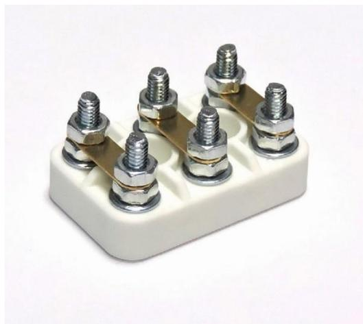
These terminals allow the connection star-delta three-phase motors or two separate motors. Thanks to the excellent thermal resistance properties conferred by ceramics, they find application in machinery such as electric ovens, motors with high operating temperatures, equipment where very high temperature resistance is required, such as smoke and heat extraction fans. These terminal blocks are also used for star-delta switching of three-phase heaters.
